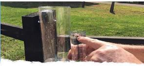
1.USE INNER TUBE TO MEASURE RAINFALL 2.POUR ANY RAIN COLLECTED IN THE OUTER TUBE THROUGH FUNNEL INTO INNER
